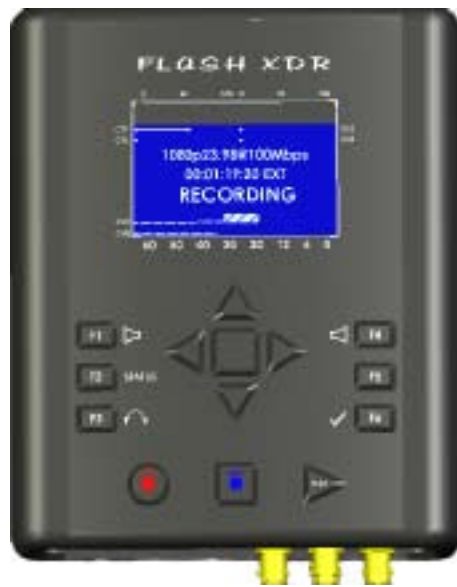
Top View LCD Panel, Function Keys, Status LEDs, Record, Stop, Play
