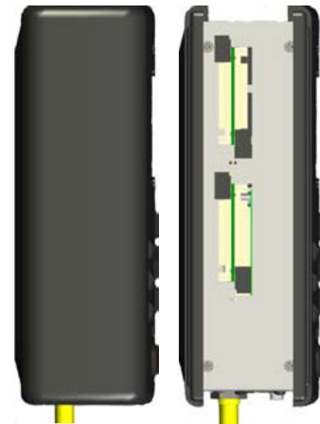
Left Side Compact Flash Slots With and Without Cover
