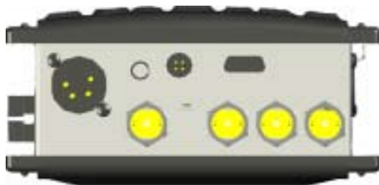
End View Power In (XLR), HP Out, GPIO, RS-422, On/Off TC I/O, 1394, SDI Out, SDI/ASI Out, SDI/ASI In
